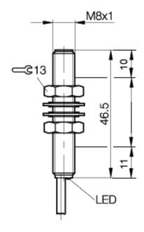
Inductive Sensors BES 516-324-G-E4-C-02 M8x1 x 30 normally-open Sn=2mm shielded
